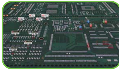
More Intuitive Defective Pads Display
